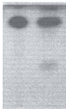
Fig. 1. Evidencing of synthesis product(s) in comparison with aglycon. Lane 1, D,L- \alpha -tocopherol; lane 2, mixture of D-galactofuranosylation products. Migration, SS 1 (toluene-methanol, 7/1, v/v). Visualisation, mostain
