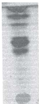
Fig. 8. Three glycosides were produced, separated and characterized by cholesterol glycosylation [29]. Migration, SS 2, chloroform-methanol-water, 50/10/1, v/v. Visualization, mostain
