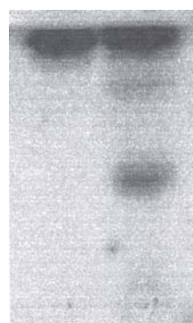
Fig. 2. Separation of thiamine D-(2,3,5,6-tetra-O-benzoyl) galactofuranoside (faster moving compound) of unreacted thiamine. Migration, SS 5 (acetone-n-butanol-water, 5:4:1, v/v); Visualisation, mostain
